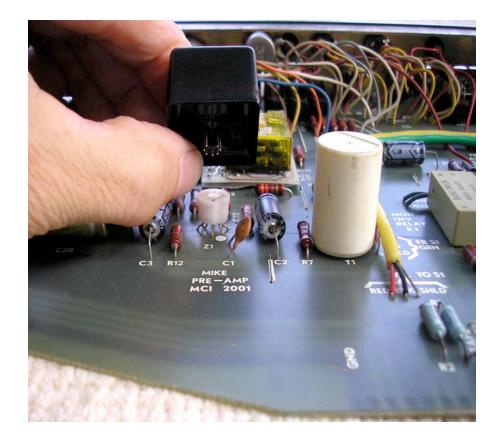
When oriented properly, opamp pins 1 and 7 will straddle unused pin hole 8 on the socket.
